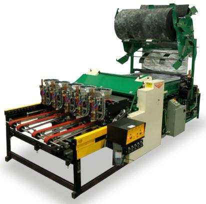
The VICON Automatic Duct Liner Application System automates the processes of unwinding, cutting, applying adhesive to sheet metal, and securing duct liners without needing tooling or blade changes. It accommodates various liners like Armaflex® and K-Flex®. An optional four-position insulation coil holder further reduces downtime during insulation changeovers for long or short runs.
