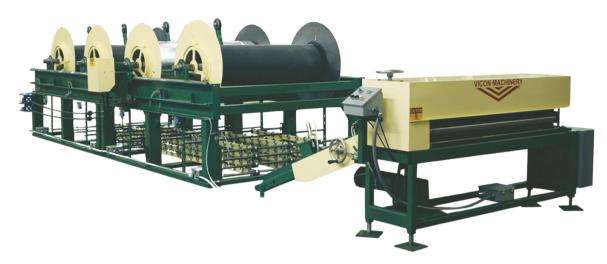
Optimize your operations and cut costs with the Vicon Coil Feeding System. Designed to streamline your workflow, this advanced system reduces waste and eliminates manual labor by uncoiling, straightening, beading, and feeding materials of varying thicknesses directly to your laser or plasma cutting machine.
