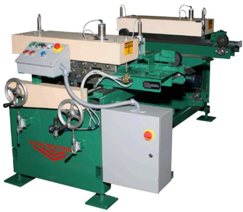
The VICON Dual Head Cleat Edge Former rollforms a 7/16" cleat edge on both ends of the duct after the Male and Female lockseam has been rollformed.
