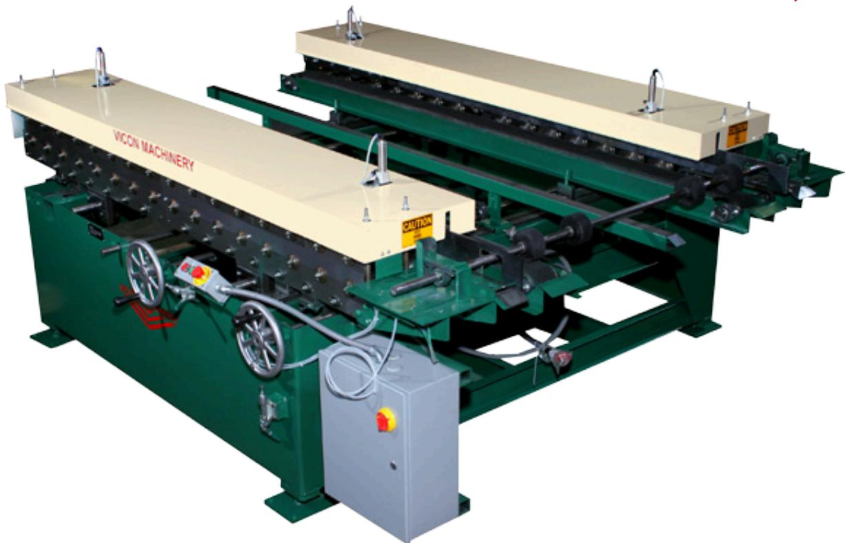
The VICON TDX Dual Head Rollformer is designed to produce your preference of either T-25a or T-25b SMACNA approved transverse flange connector.
