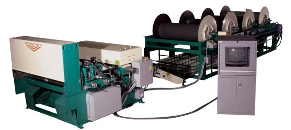
The VICON duct fabrication system centers around the essential Duct-Line Express front-end. Transform it into a complete Full Coil Line effortlessly by integrating modular VICON Coil Line components, delivering exceptional versatility and productivity.
