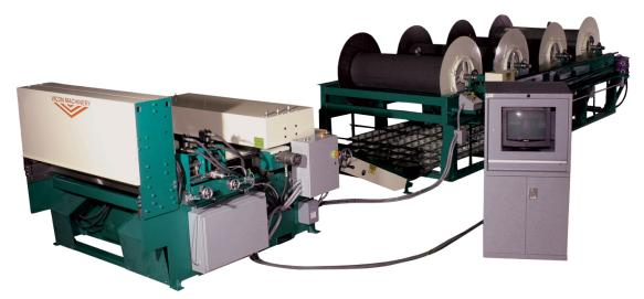
The VICON duct fabrication system centers around the essential Duct-Line Express front-end. Transform it into a complete Full Coil Line effortlessly by integrating modular VICON Coil Line components, delivering exceptional versatility and productivity.
