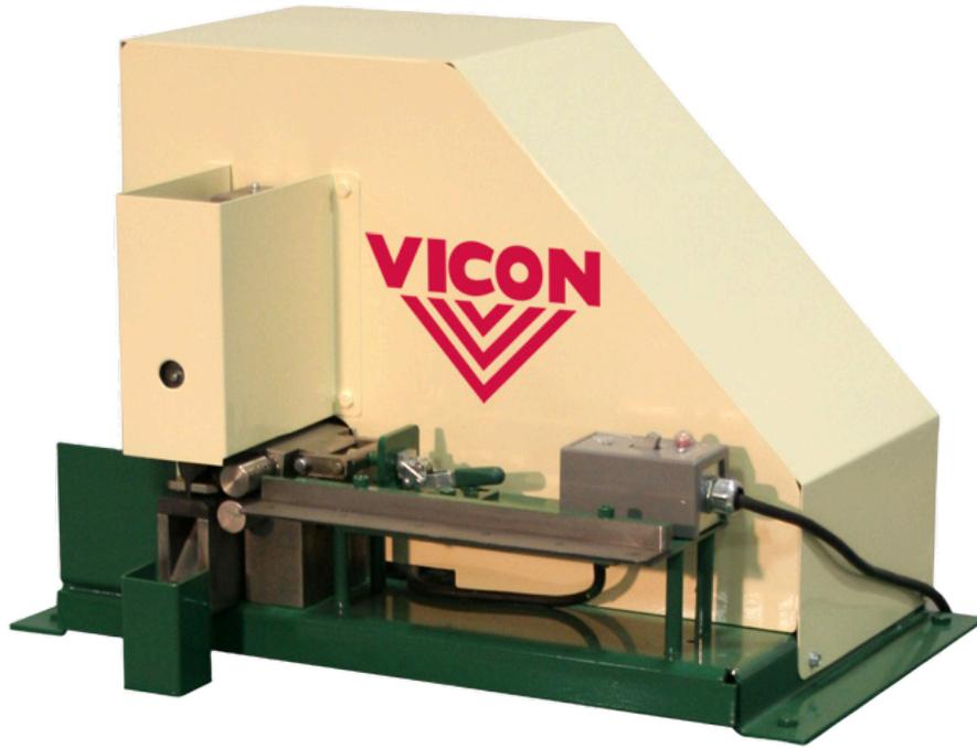
The Vicon Edge Notcher includes a feature for releasing the latch, allowing notching of round pipes after they have been rolled. It is also capable of notching tap-in locks after they have been roll formed. By adjusting the guide depth, the punch can notch right up to the standing seam profile. The notch pattern can be performed in the flat, prior to rollforming.
