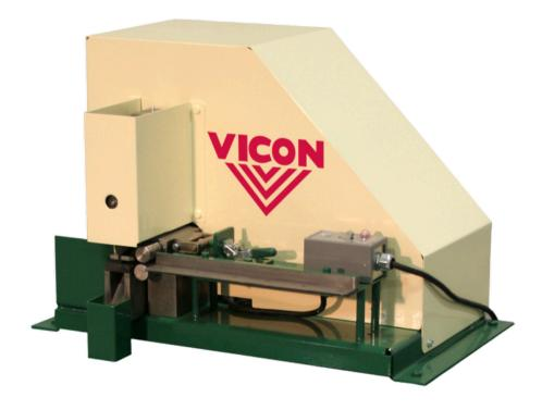
The Vicon Edge Notcher includes a feature for releasing the latch, allowing notching of round pipes after they have been rolled. It is also capable of notching tap-in locks after they have been roll formed. By adjusting the guide depth, the punch can notch right up to the standing seam profile. The notch pattern can be performed in the flat, prior to rollforming.
