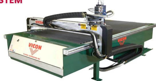
The Vicon Fabricator SS is a rugged and flexible plasma cutting machine. The solution for the optimal processing of fabrication or job shop applications. With its swift, precise, and clean CNC cutting capabilities, this system significantly minimizes waste and operational expenses, leading to greater profitability.
