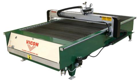
This robust and adaptable machine provides an ideal solution for effectively processing HVAC duct fittings. Fast, accurate, and efficient, this CNC cutting system greatly reduces material waste and operational costs, resulting in enhanced profitability.
