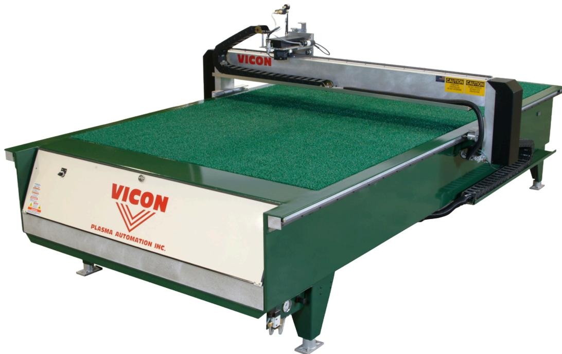
An economical stand-alone machine, the HVAC 510SL is dedicated to cutting acoustical liner in low and high volume shops. It is the ideal solution for users with existing plasma cutting systems that need additional liner cutting capability.
