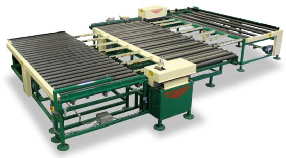
The VICON Lockseam System excels in design, providing a user-friendly and reliable method for automatically creating Pittsburgh and Snaplock seams. Its "Accessible Concept" eliminates overhead devices to minimize miss-feeds or jams, while the "open top" feature allows for larger blanks to be fed into the TDX, liner, and brake systems.
