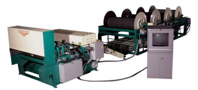
**PIPE-LINE EXPRESS -** The Pipe-Line Express includes an uncoiler (patented), feeder, straightener unit, beader, notching unit and heavy duty shear.
