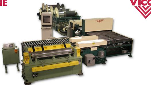
Dependable performance, impressive productivity, and outstanding part transfer are just the beginning. The Vicon Pipe Line is designed to manufacture precision round pipe sections at remarkable speed. It can handle sizes from 3 inches to 24 inches in diameter, using either the Reeves or modified lock seam. This innovative pipe line is engineered to create highly profitable ductwork.
