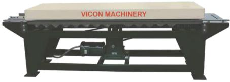
The Vicon TDX 16 Station Rollformer is specifically designed to produce the T-25a transverse flange (four-bolt) connection. This profile has been rigorously evaluated by the SMACNA Testing and Research Institute and meets the criteria outlined in SMACNA's HVAC Duct Construction Standards.
