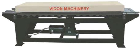
The Vicon TDX 16 Station Rollformer is specifically designed to produce the T-25b transverse flange (four-bolt) connection. This profile has been rigorously evaluated by the SMACNA Testing and Research Institute and meets the criteria outlined in SMACNA's HVAC Duct Construction Standards.
